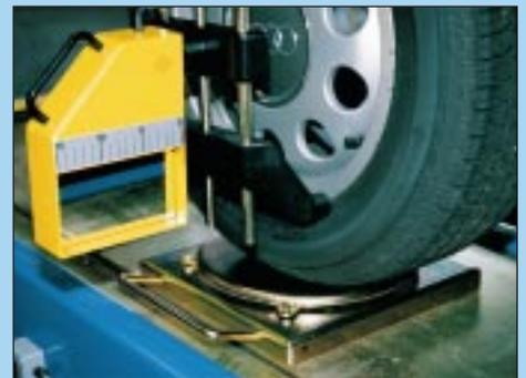
Twin Scale System for measuring on rear wheels.
