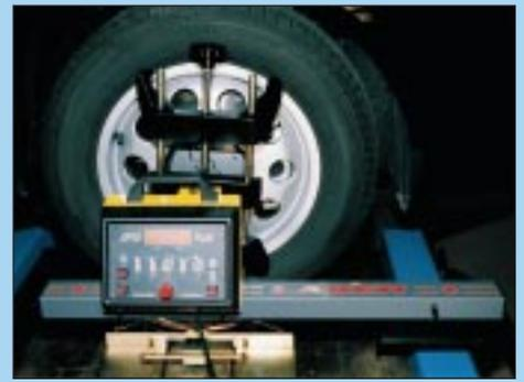
Front panel for measuring Camber, Caster, King Pin & Caster Adjustment.
