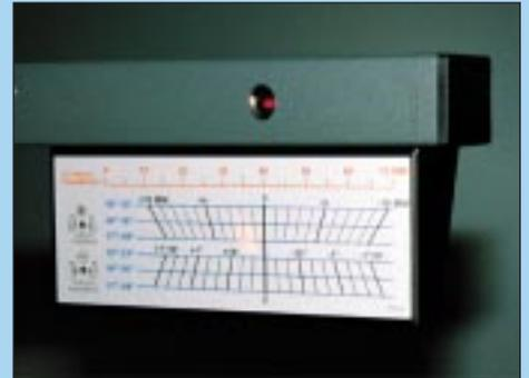
Toe scale projected for measuring Toe and Set Back.
