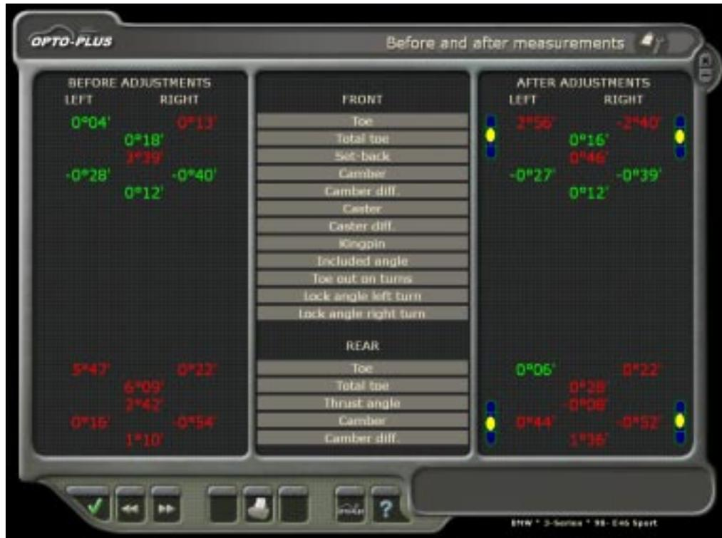
All stored values inside tolerance are shown in green, values outside tolerance are shown in red, while values without manufacturer specifications are shown in grey.
