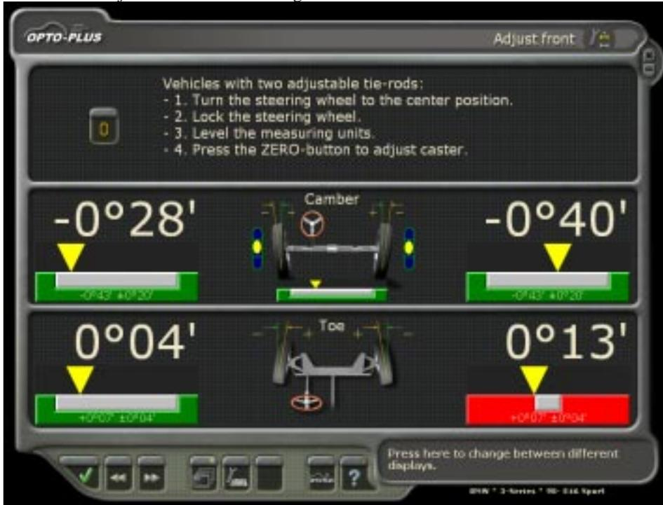
To adjust caster it is necessary to initiate the correct measuring conditions as described on the screen.
