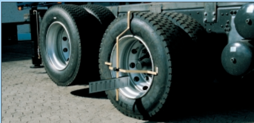
With the self centering frame check tool 039400 and 040100, the chassis and axles can be easily checked
